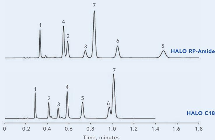
Hydrogen bond donors, like 2-chlorophenol, 3-ethylphenol, and butyl paraben are more strongly retained on the HALO RP-Amide phase than on the HALO C18 phase. Basic compounds, like N, N-dimethylaniline, are slightly less retained on the HALO RP-Amide phase. This difference in selectivity makes HALO RP-Amide an extremely useful alternate selectivity to the HALO C18 phase.
