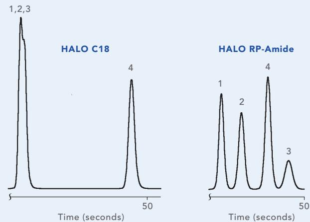
Three compounds in this sample mix do not separate on a C18 phase. Under identical mobile phase conditions, they are baseline separated on the HALO RP-Amide.
