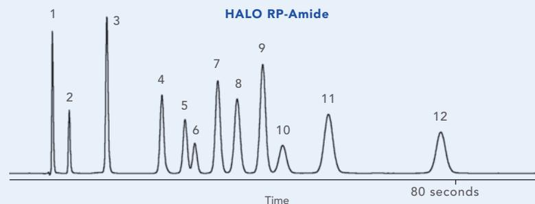
The selectivity offered by the alkyl amide phase combined with the high efficiency and high speed of the HALO Fused-Core particles facilitates the separation of these 12 compounds in under 80 seconds.
