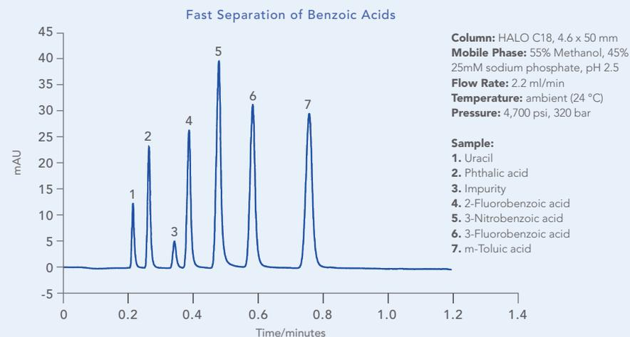
HALO columns are designed for hyper-fast separations so that higher sample throughput can be achieved. In this example, the HALO column separated seven compounds in less than 48 seconds with better than baseline resolution for all peak pairs.
