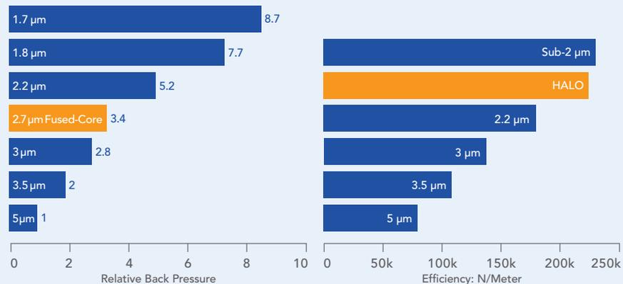
HALO columns packed with Fused-Core particles provide over 80% of the efficiency (theoretical plates, N) and 90% of the resolving power of sub-2-μm columns, but require less than half the back pressure. This lower pressure permits HALO columns to be used with conventional 400 bar-limit HPLC equipment and achieve speed and resolution very similar to UHPLC.
