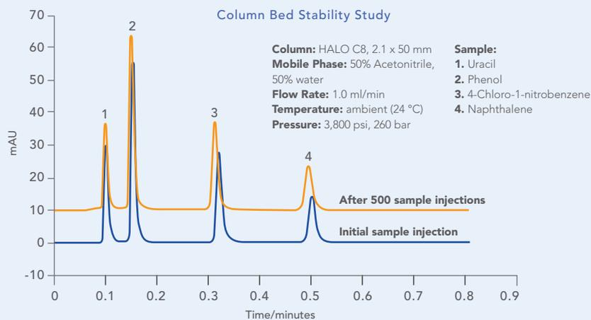
A HALO column was run under high flow conditions to test bed stability. After 500 sample injections and over 40,000 column volumes, there was no evidence of any change to the packing bed.
