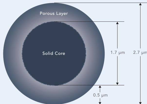
Fused-Core particle technology was developed by Jack Kirkland to produce HPLC columns that provide faster separations and higher sample throughput without sacrificing column ruggedness and reliability. As the name implies, Fused-Core particles are manufactured by “fusing” a porous silica layer onto a solid silica particle.
