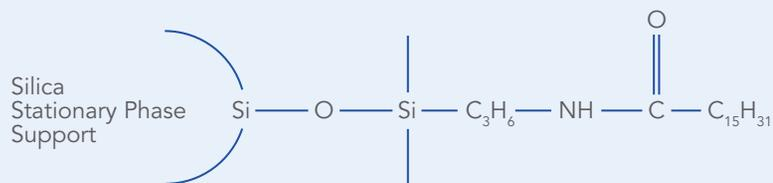
A stable amide group embedded in an 18-carbon chain is the bonded phase used for the HALO RP-Amide phase.
