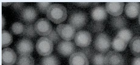
This SEM photograph of HALO particles illustrates two important attributes of this unique column packing. First, the incredibly narrow particle size distribution is apparent. Second, this SEM photo shows some of the HALO particles “sliced in half” so that the solid core and the porous outer layer, the “halo” of the particles, is evident.
