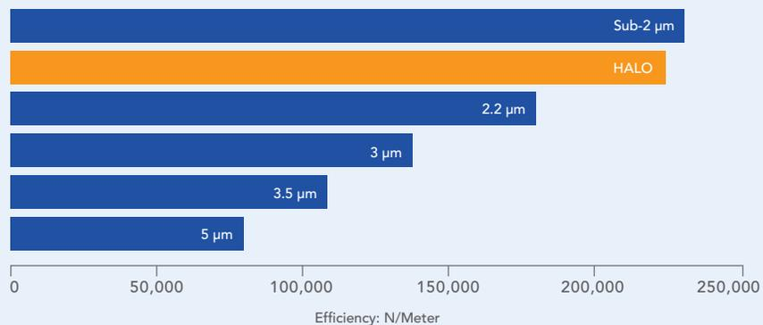
HALO columns deliver over 90% more separating power (theoretical plates) than columns of the same length packed with 3.5 μm particles and almost three times the separating power of columns packed with 5 μm particles.
