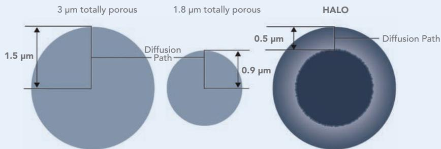
The shorter diffusion path of HALO particles reduces axial dispersion of solutes and minimizes peak broadening. Because of the shorter diffusion path, the performance advantages of HALO become even more apparent when separating larger solute molecules and operating at faster mobile phase flow rates.
