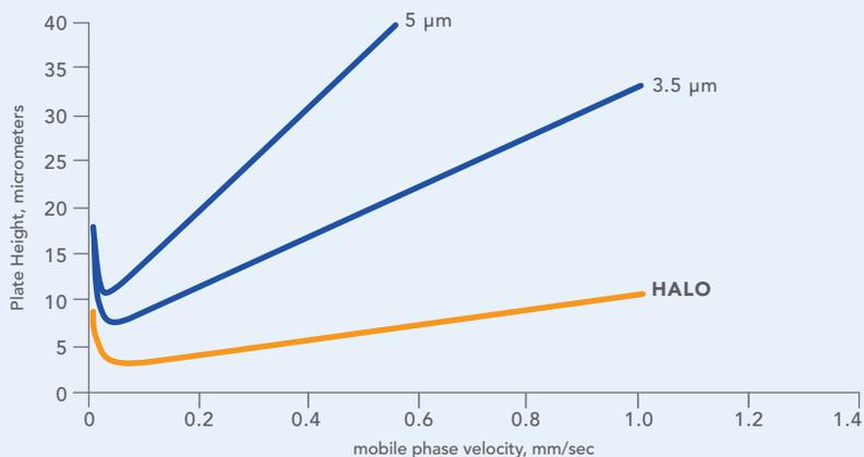
Van Deemter plots are a convenient way to compare the efficiency of HPLC columns. In this comparison we see that HALO columns are more efficient than columns packed with 5 μm or 3.5 μm particles and that they can be run at higher mobile phase linear velocity and still maintain their resolving power.
