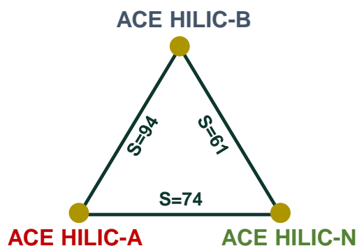
Figure 2 Selectivity triangle for the ACE HILIC range using HILIC probes on 10 mM ammonium formate pH 4.7 MeCN/H 2 O (90:10 v/v)
