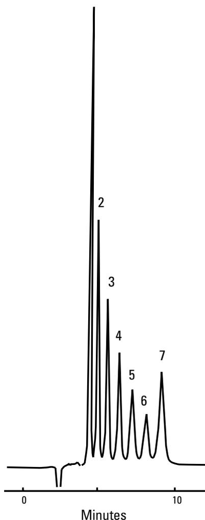
Column: TSKgel Amide-80 (4.6 mm ID x 25 cm L); Sample: 2  $\mu$ L,  $\beta$ -cyclodextrin hydrolysate, 1 - 7 degrees of polymerization (4.6 mg/mL); Elution: ACN/water (55/45); Flow Rate: 1.0 mL/min; Detection: RI; Temperature: 25  $^{\circ}$ C
