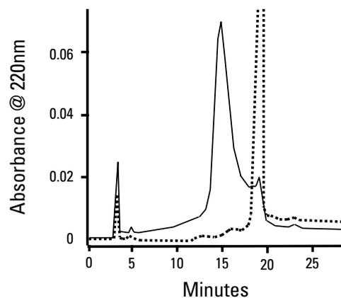
Column: TSKgel Ether-5PW, 7.5 mm ID x 7.5 cm L; Sample: C-1027, C-1027-AG concentration: 1 mg/mL; Injection: 20  $\mu$ L; Elution: linear gradient from 1.5 mol/L to 0 mol/L  $(\text{NH}_4)_2\text{SO}_4$  in 0.1 mol/L phosphate buffer, pH 7.0; Flow Rate: 0.8 mL/min; Detection: UV@220nm
