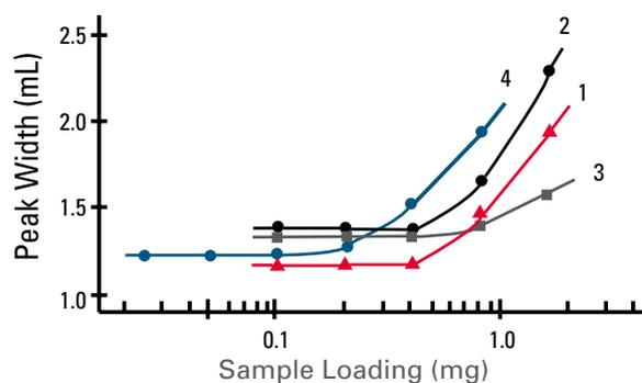
Column: TSKgel Phenyl-5PW, 7.5 mm ID x 7.5 cm L; Sample: 1. myoglobin; 2. ribonuclease A; 3. ovalbumin; 4. α-chymotrypsin; concentration: 0.025 % to 1.6 %; Elution: 60 min linear gradient of (NH<sub>4</sub>)<sub>2</sub>SO<sub>4</sub> from 1.5 mol/L to 0 mol/L in 0.1 mol/L phosphate buffer (pH 7.0); Flow Rate: 0.5 mL/min; Temperature: 25 °C; Detection: UV@280 nm
