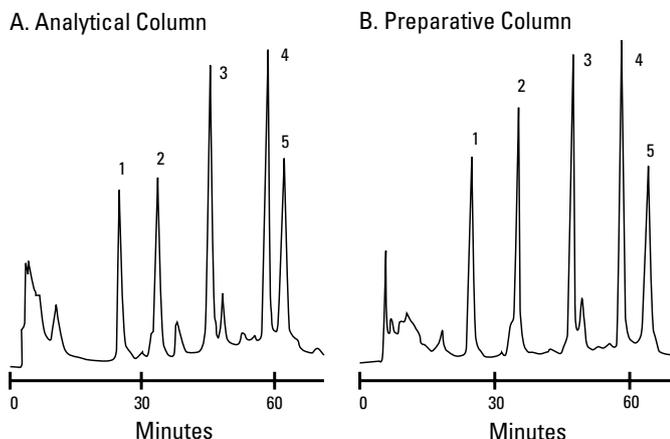
Column: TSKgel Phenyl-5PW, A.) 7.5 mm ID x 7.5 cm L and B.) 21.5 mm ID x 15 cm L; Sample: 1. myoglobin, 2. ribonuclease A, 3. lysozyme, 4. α-chymotrypsinogen, 5. α-chymotrypsin; Elution: 60 min linear gradient from 1.8 mol/L to 0 mol/L (NH<sub>4</sub>)<sub>2</sub>SO<sub>4</sub> in 0.1 mol/L phosphate buffer, pH 7.0; Flow Rate: 0.5 mL/min (7.5 mm ID) or 4 mL/min (21.5 mm ID); Detection: UV@280nm
