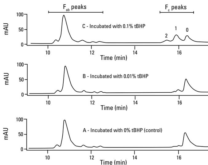
Column: TSKgel Butyl-NPR, 4.6 mm ID x 3.5 cm L; Elution: Buffer A: 2 mol/L (NH<sub>4</sub>)<sub>2</sub>SO<sub>4</sub>, 20 mmol/L Tris, pH 7, Buffer B: 20 mmol/L Tris, pH 7; Gradient: linear from 10 % B to 100 % B in 34 minutes; Flow rate: 1 mL/min; Temperature: 30°C
