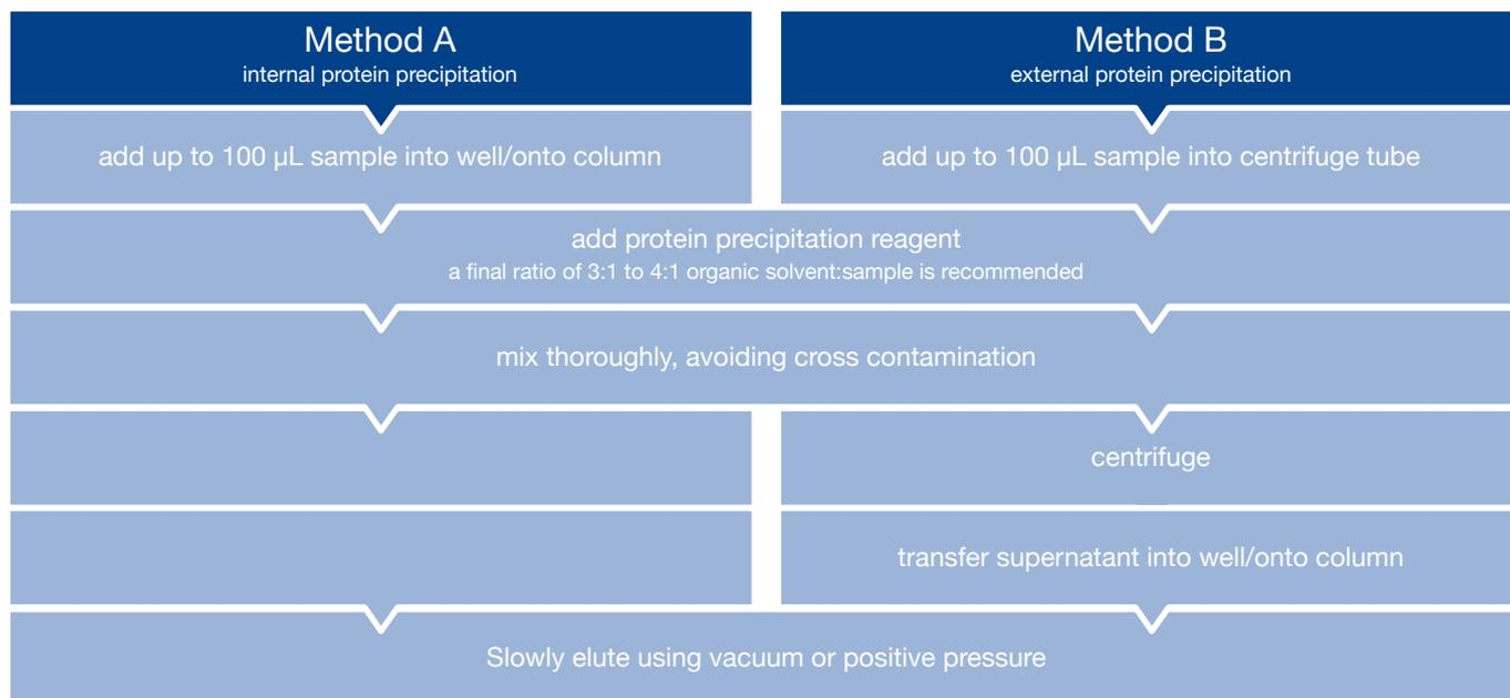
CHROMABOND® PL products are designed for internal protein precipitation (method A). External protein precipitation (method B) could be necessary in order to prevent upper frit and adsorbent bed clogging due to the nature of precipitated proteins. The choice of the protein precipitation reagent depends on the application.
