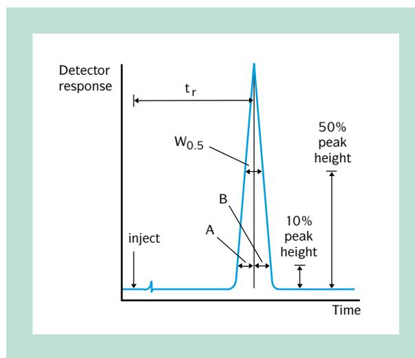
Figure 16 | Measurement of peak efficiency and peak asymmetry.
