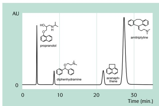
**Figure 7 | Separation of propranolol, diphenhydramine, acenaphthene and amitriptyline.**
