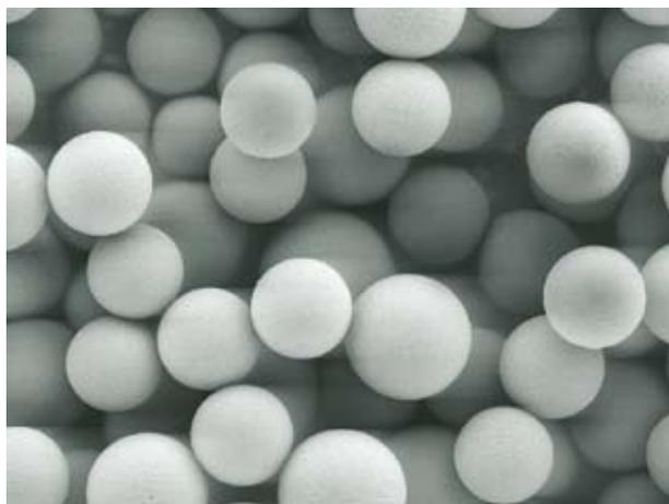
Figure 1 | FE-SEM image of Kromasil 100 Å, 3.5 μm particles.
