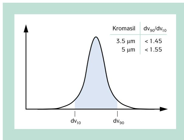
Figure 2 | Particle size distribution showing the  $dv_{90}/dv_{10}$  ratio.
